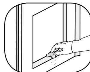
Smooth out any rough edges with sand paper. Refer to Quick Start Guide for fitting.
